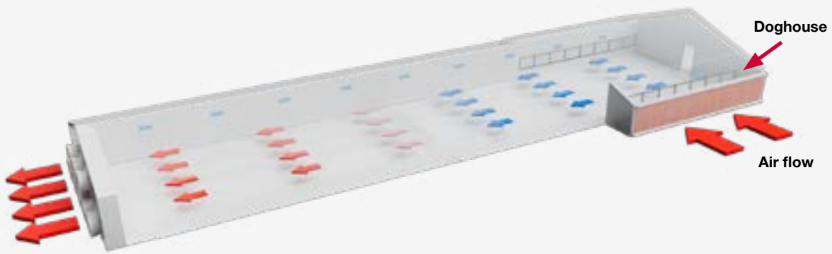
Figure 6.18 Air flow in a tunnel-ventilated house.
