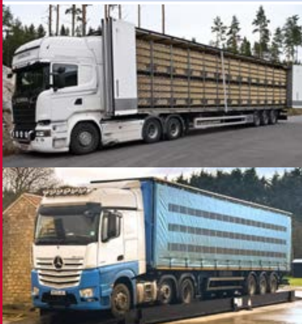
Figure 4.5 Examples of vehicles suitable for transporting broilers to the processing plant.
