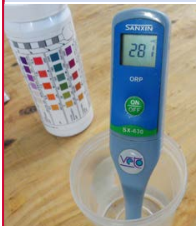
Figure 7.6 An example of an ORP meter.
