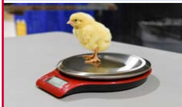
Figure 3.8 Electronic platform scales for individual bird weights up to 7 days of age.
